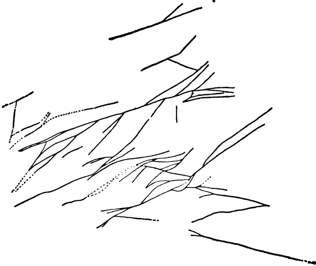
Fig. 46. Linked veins. Surface plan of vein system of Pachuca, Mexico. Scale 1—50,000. After E. Ordoñez.
